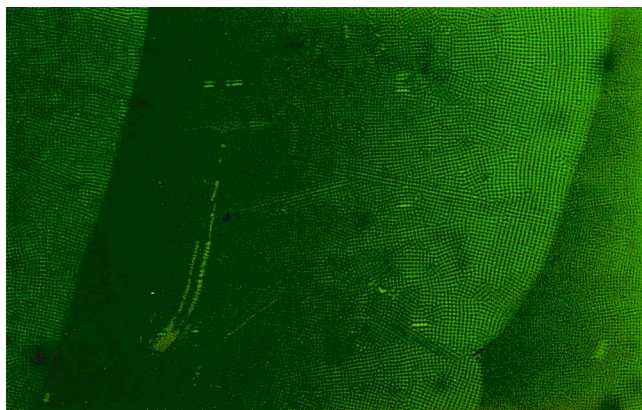
Figure 2. Photomicrograph (magnification \times 320 ) obtained for the UTGBC* phase at 201.4°C while cooling from the TGB phase of trimesogen 2 . The sample was placed in a wedge-type cell with the glass plates treated for planar orientation. Notice the Grandjean Cano dislocation lines superposed on the square grid pattern.
